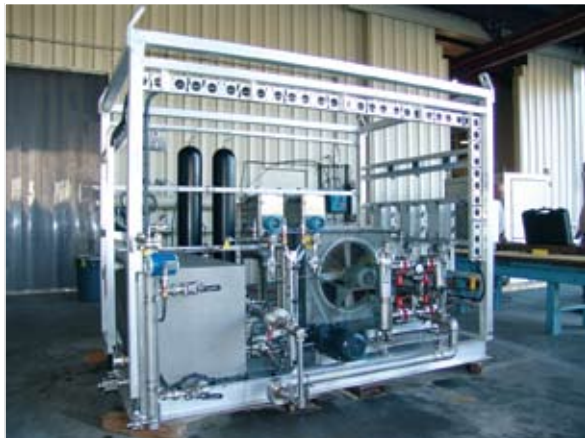
HPU/Lube Oil Skid
